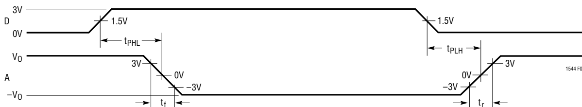
Figure 8. V.10, V.28 Driver Propagation Delays
